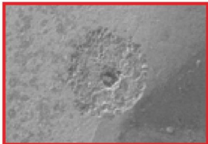
Scanning electron microscope image, chloride-induced pitting
