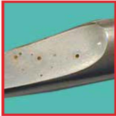
Chloride-induced pitting on instrument.
